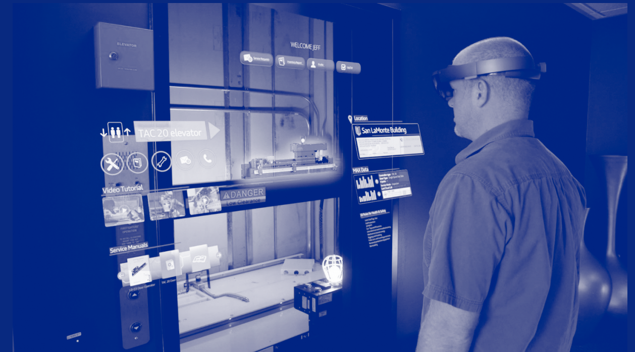
e. HoloLens users can manipulate a computer interface and 3D images only they can see with simple hand gestures. (Source: ThyssenKrupp)
